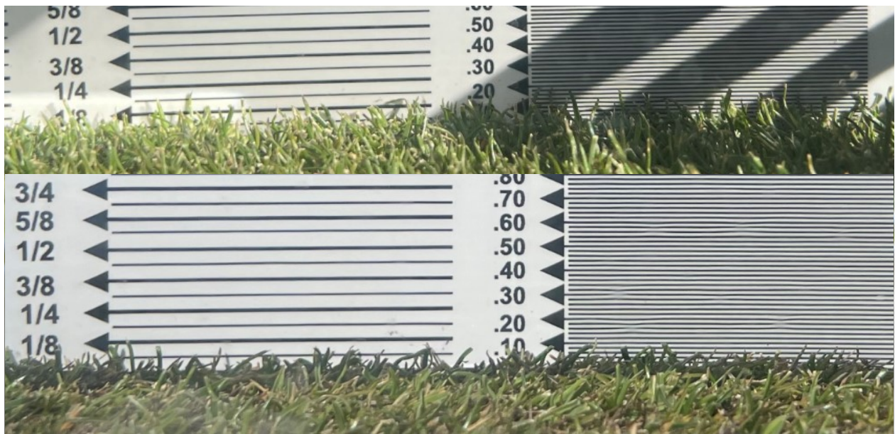
The prism gauge reads a field height of cut at about 0.170 inches (top) and much lower at about 0.120 inches (bottom).
